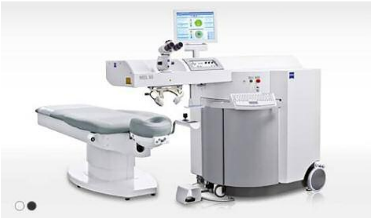
Figure 13. The Zeiss MEL-80 laser system consists of an ArF excimer laser. This is a good example of a value-added system. Used for ophthalmic surgery, the laser itself is not readily visible.
