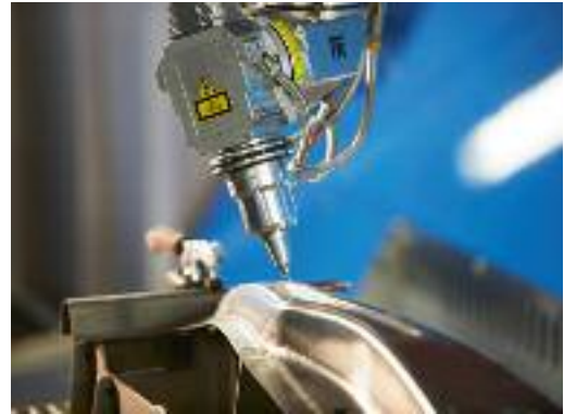
3D fiber laser cutting machine dedicated to the automotive industry
