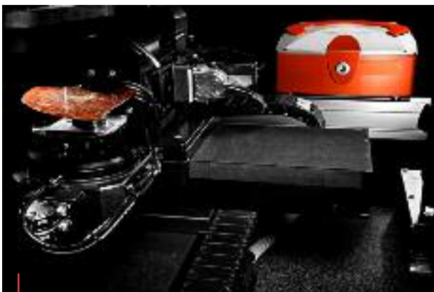
Satsuma ultrafast fiber laser used in the semiconductor and display industries
