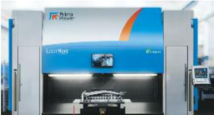
3D fiber laser cutting machine dedicated to the automotive industry
