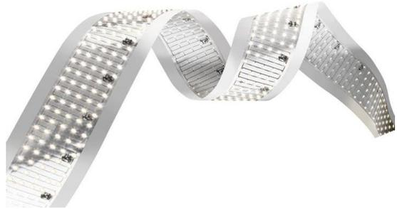
LED lighting system with width from 25 to 250 mm and length up to 2,4 m that combines mechanical, electrical and source functions together in a flexible sheet of light; high efficacy at 110 lm/W, white light CRI>80 and 50Khr life.
