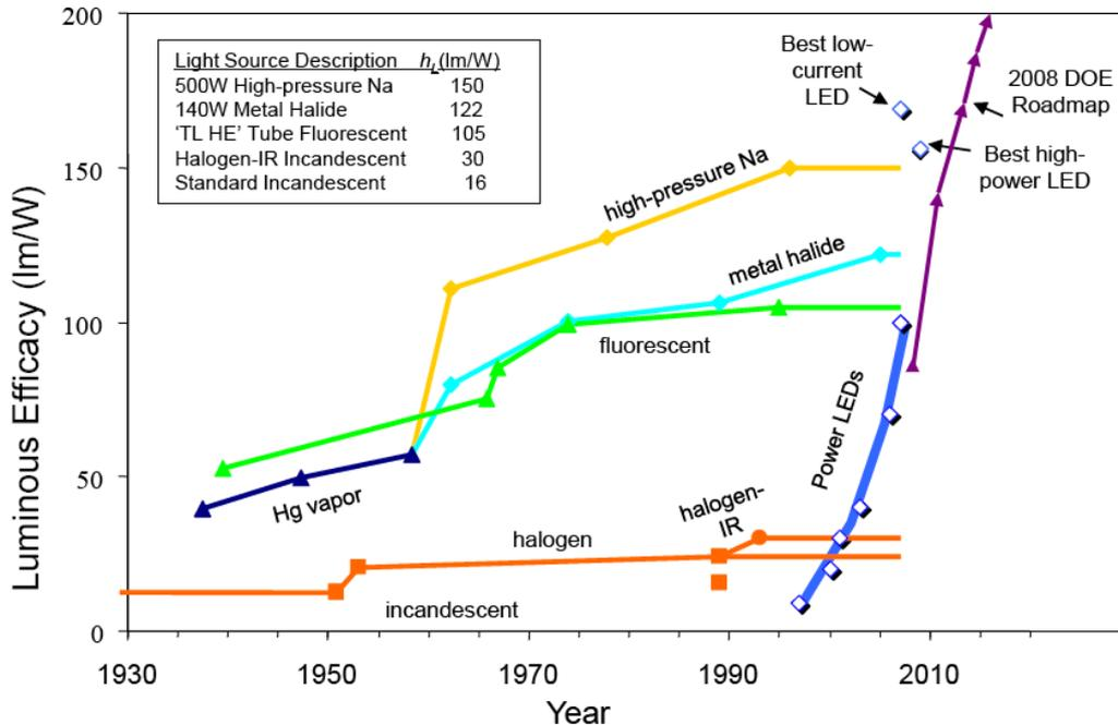
Fig.2: Efficacy evolution of best-in-class LEDs; comparison with discharge lamps
