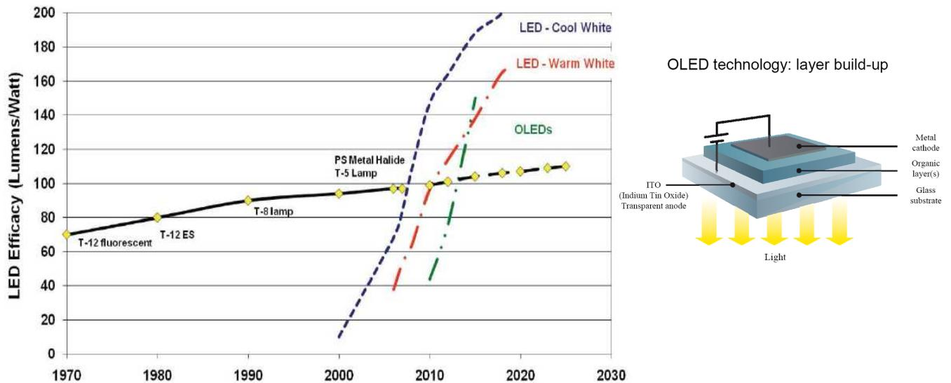
Fig.5: Efficacies of OLEDs compared with those of LEDs
