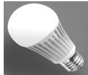
ULTRA LED Retrofit A-line Lamps 6W (50 LPW, 3000K) 8W (54 LPW, 3000K) 12W (67 LPW, 2700K) by OSRAM Sylvania
