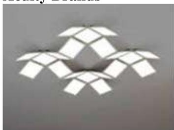
A 5-panel modular OLED ceiling mounted system of 6.5 watt, 4" square panels at 60 lumen per watt and CRI = 85.
