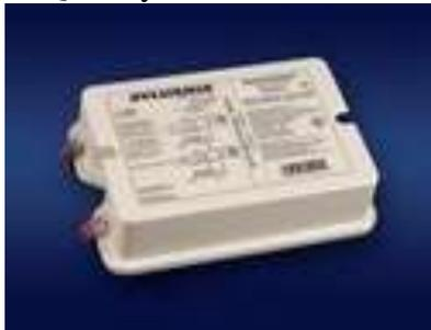
A UL Type II wet location, high efficiency HID 50% step-dimming ballasts for standard 100 to 200 watt MH and HPS lamps.
