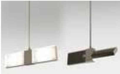
A 10 or 20 watt single or double 12 volt wall wash track head producing 600 or 1200 lumen dimmable to 10% in flood or asymmetric optics.
