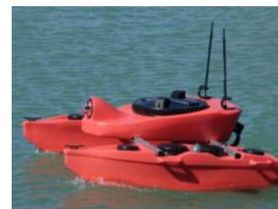
SWAP: Aquatic drone for integrated monitoring of marine and lagoon ecosystems
