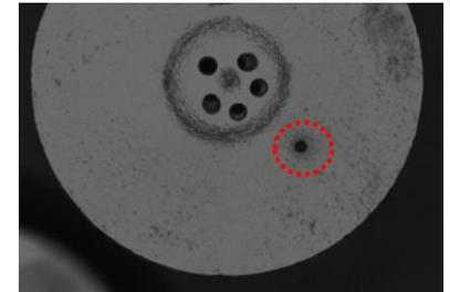
c) Align "spray-hole" with "step-hole"
