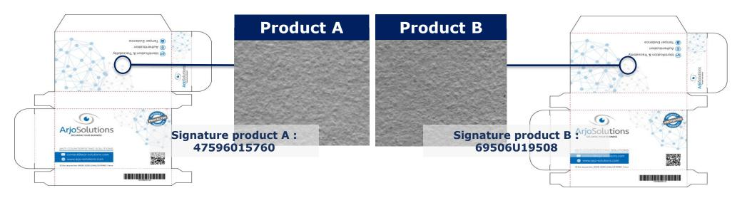
As for **human's digital fingerprints**, two products can be differentiated based on the unicity of the hazards visible on a material Our solution converts via our **patented**, **proprietary digital fingerprinting algorithm**, these visible hazards into a **unique digital signature of the product**
