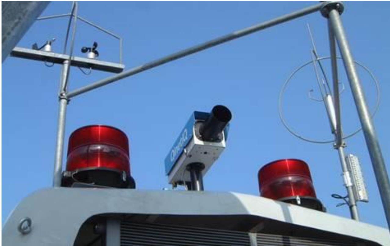
Zephir prototype on a Nordex N90 turbine nacelle, 4 March 2003
