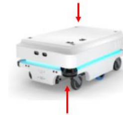
Sensors positioned cornerwise on an AMR
